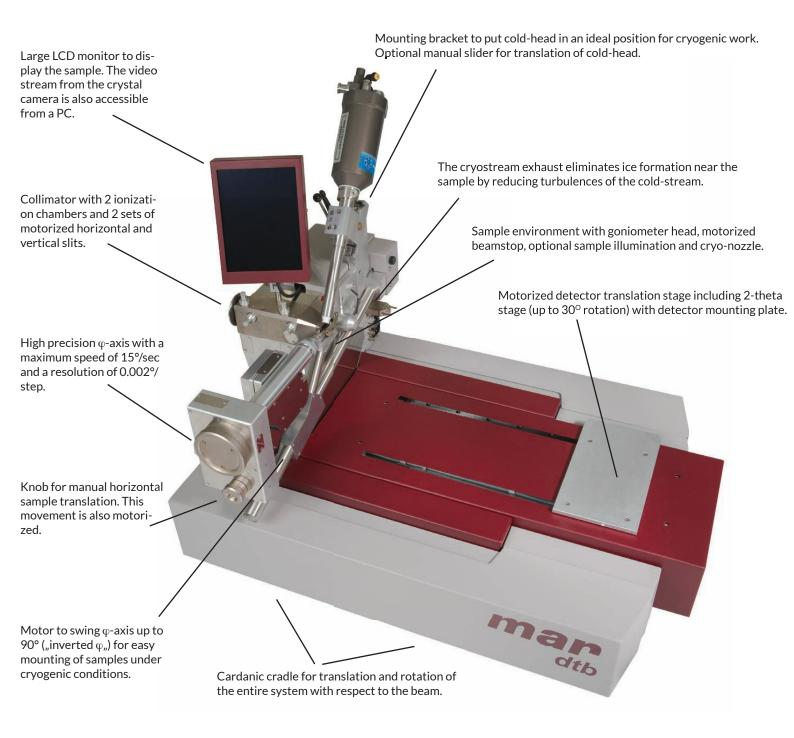
The **mar** dub is a highly versatile goniometer system for general use in X-ray crystallography. Due to an autonomous control system, it can accomodate any X-ray detector, e.g. the **mar** 345 image plate or the family of CCD-detectors produced by Rayonix
